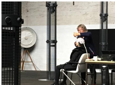
Figure 1: E1 EEG measurements by Dr. Anat Barnea from the BioKeshev Institute at MONOM Center for Spatial Sound Berlin. The omnidirectional speakers are placed in the observed black columns. Each column holds 3 speakers: at ground level, top (4 m) and middle.
